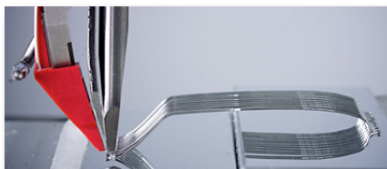
Loop Former option enables advanced square shaped loop profiles
