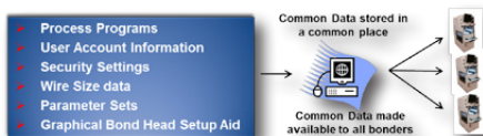
Bonder Data such as user accounts, security settings, bond parameter sets and wire size data can be transferred from a host to all machines to ensure commonality and production line control
